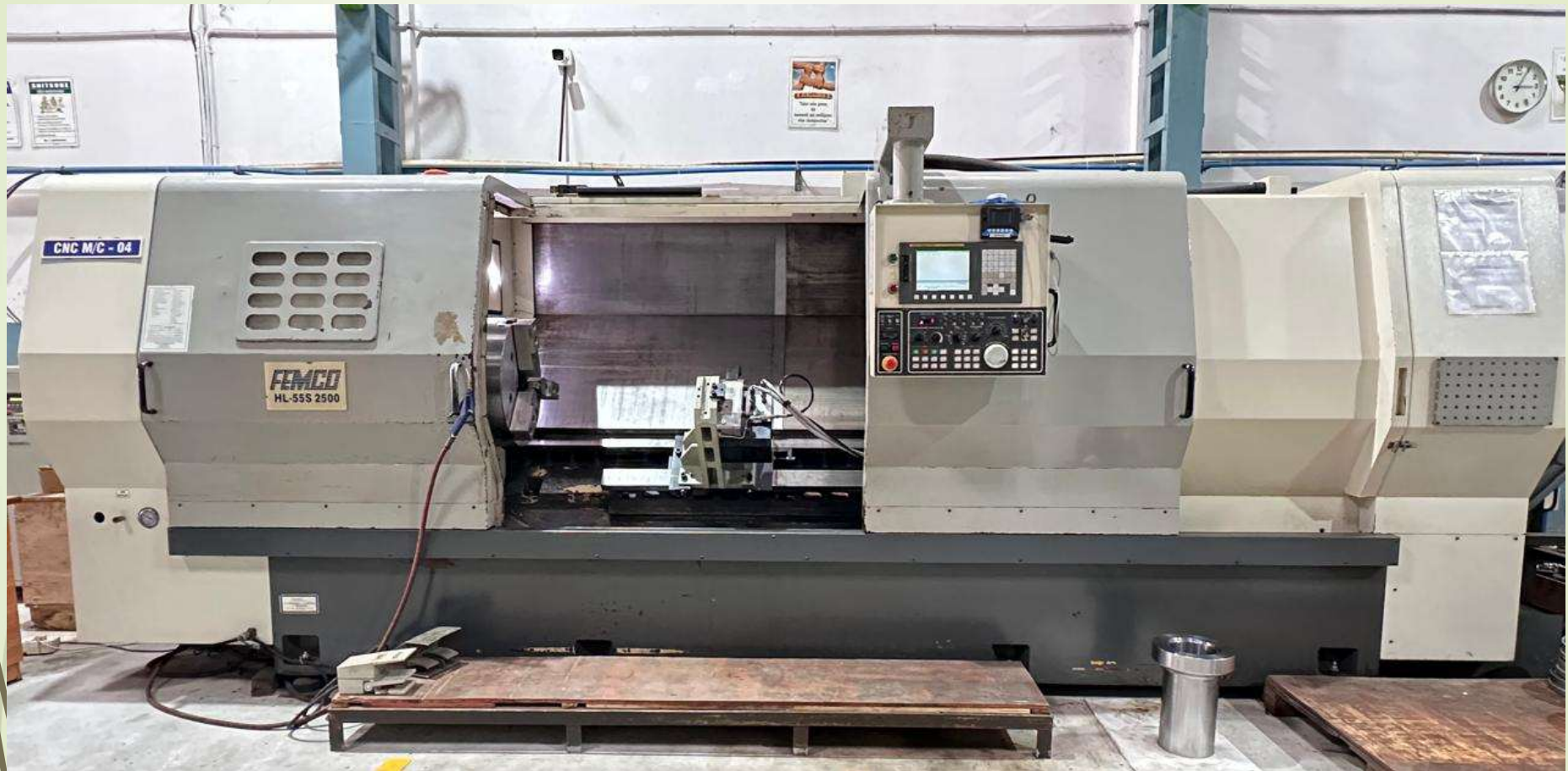
CNC MACHINE-04 CAPACITY: Ø - 400 mm, L - 2320 mm MAKE: FEMCO
